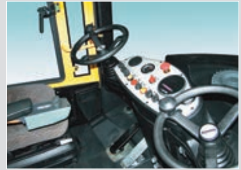
Two steering positions with a sliding seat makes the work environment more comfortable and safe.
