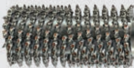
Fine milling drum Milling width: 2,000 mm Milling depth: 0-100 mm Tool spacing: 8 mm
