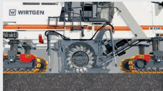
2 | Cold milling machine is lowered quickly while retaining its parallel alignment
