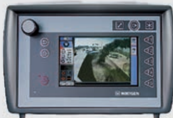
2 | Camera at end of conveyor
